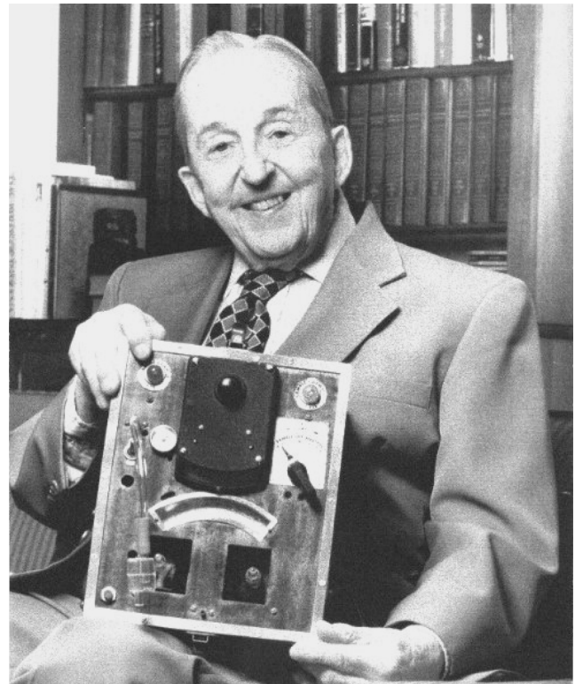
Professor Borkenstein (photo taken 1996) holding the first hand-made version of the Breathalyzer.
